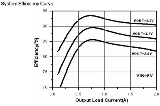
Figure 5. XL1410 System Efficiency Curve
