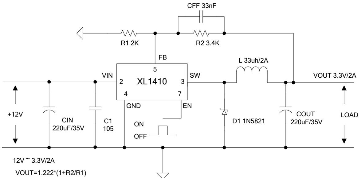
Figure8. XL1410 System Parameters Test Circuit (12V ~ 3.3V/2A)
