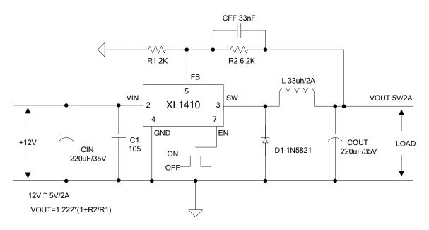
Figure 7. XL1410 System Parameters Test Circuit (12V ~ 5V/2A)
