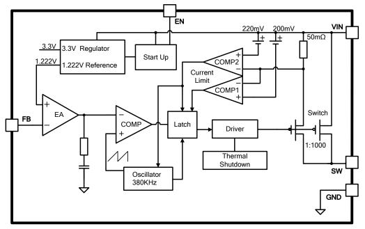
Figure 3. Function Block Diagram of XL1410
