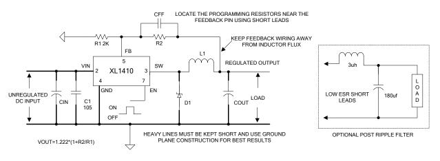
Figure6. Standard Test Circuits and Layout Guides
