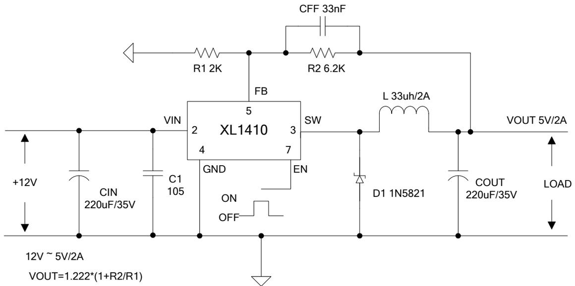
Figure7. XL1410 System Parameters Test Circuit (12V ~ 5V/2A)
