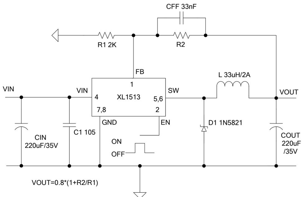
Figure4. XL1513 Typical Application Circuit
