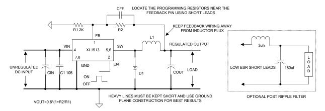
Figure 6. Standard Test Circuits and Layout Guides
