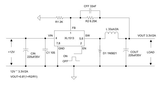
Figure 8. XL1513 System Parameters Test Circuit (12V ~ 3.3V/2A)
