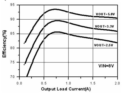
Figure 5. XL1513 System Efficiency Curve
