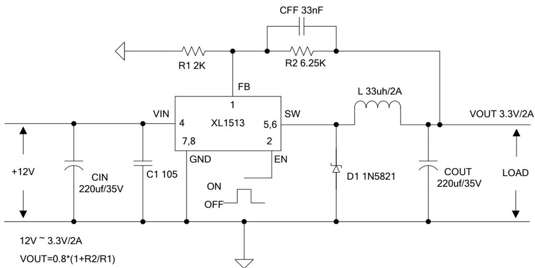
Figure8. XL1513 System Parameters Test Circuit (12V ~ 3.3V/2A)
