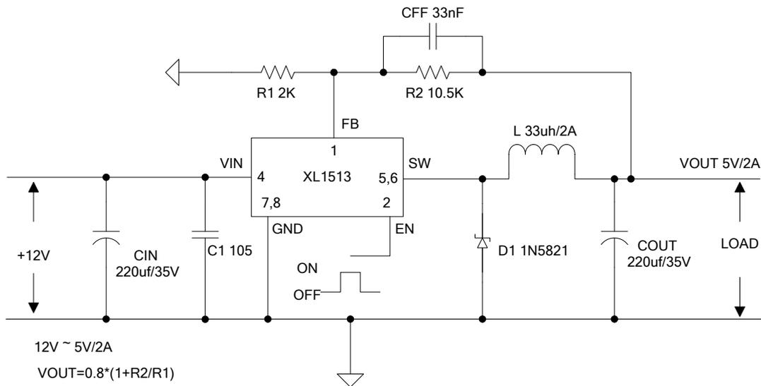
Figure7. XL1513 System Parameters Test Circuit (12V ~ 5V/2A)
