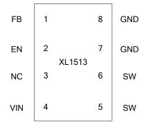
Figure 2. Pin Configuration of XL1513 (Top View)
