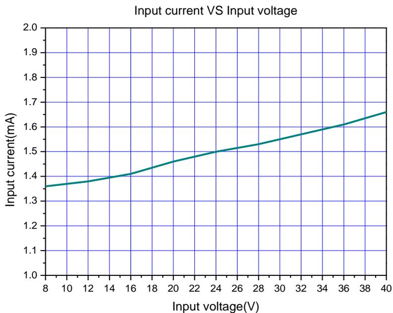
Figure9. The input current curve when output short happen.
