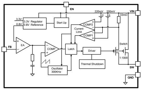
Figure 3. Function Block Diagram of XL4003
