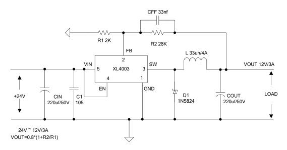
Figure 6. XL4003 System Parameters Test Circuit (24V ~ 12V/3A)
