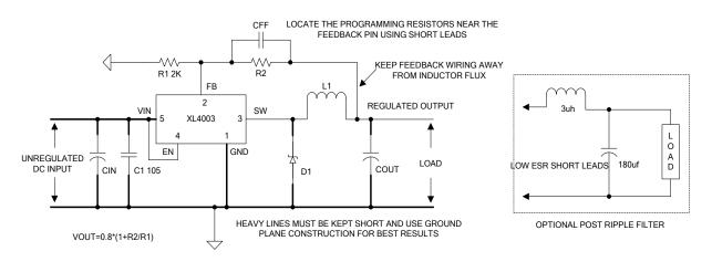
Figure 5. Standard Test Circuits and Layout Guides
