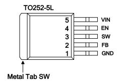
Figure 2. Pin Configuration of XL4003 (Top View)
