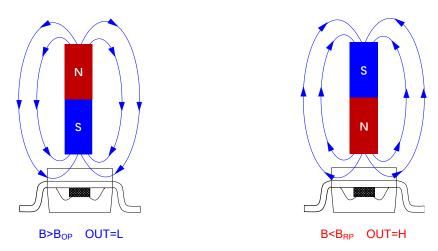
Figure 4. Magnetic Field Direction Definition
