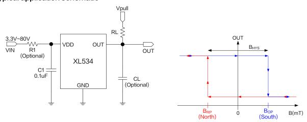
Figure 1. XL534 Typical application schematic and output characteristic curve
