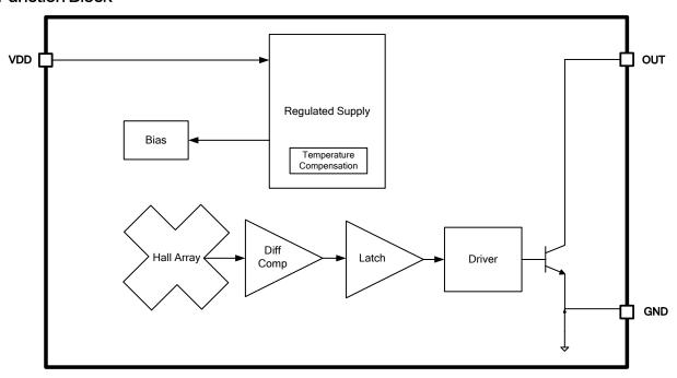
Figure 3. Function Block Diagram of XL534
