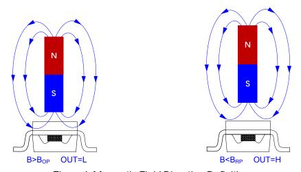
Figure 4. Magnetic Field Direction Definition
