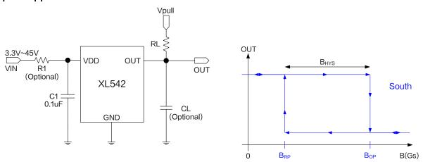
Figure 1. XL542 Typical application schematic and output characteristic curve
