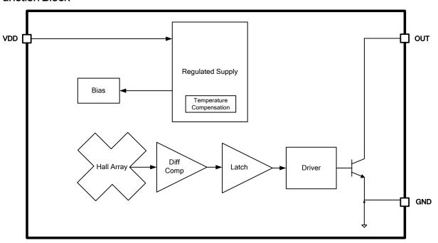
Figure 3. Function Block Diagram of XL542
