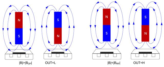
Figure 4. Magnetic Field Direction Definition
