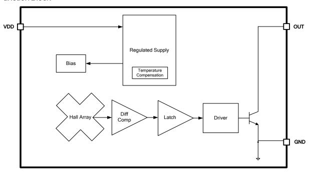
Figure 3. Function Block Diagram of XL561
