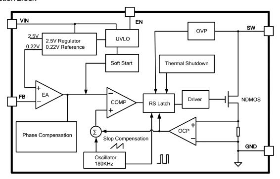
Figure 3. Function Block Diagram of XL6006
