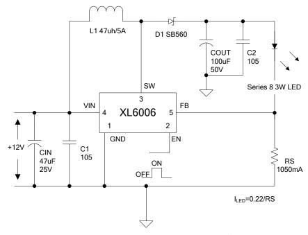
Figure 6. XL6006 System Parameters Test Circuit (12V ~ 8 x 3W LED)
