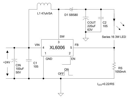
Figure 7. XL6006 System Parameters Test Circuit (24V ~ 16 x 3W LED)
