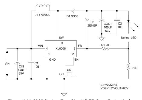
Figure 11. XL6006 System Test Circuit (LED Open Protection)
