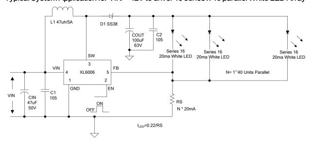
Figure 8. XL6006 System Parameters Test Circuit (VIN>=12V ~ 16 x 40 White LED)
