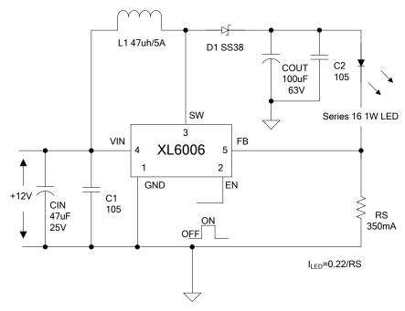
Figure 5. XL6006 System Parameters Test Circuit (12V ~16 x 1W LED)
