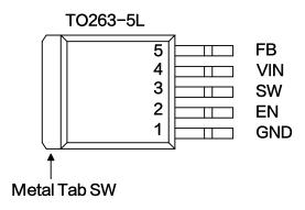
Figure 2. Pin Configuration of XL6006 (Top View)
