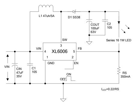
Figure 4. XL6006 Typical Application Circuit
