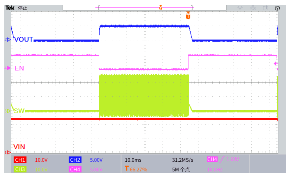
Figure36. Start or Shutdown Using EN Pin ( V_{IN}=24V , V_{OUT}=5.0V , I_{OUT}=0.5A )
