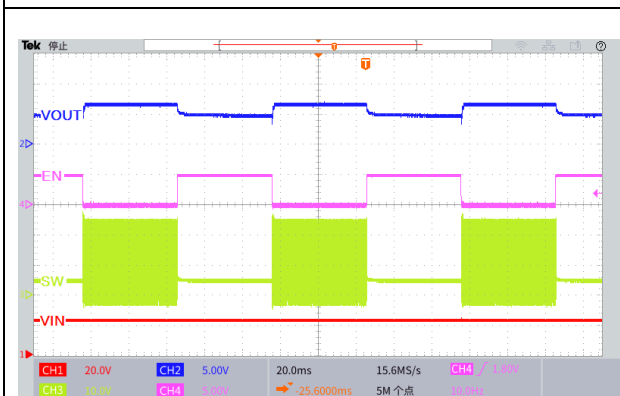
Figure33. Start or Shutdown Using EN Pin ( V_{IN}=24V , V_{OUT}=6.6V , I_{OUT}=0.3A )
