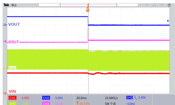
Figure22. Output Short Circuit Waveform ( V_{IN}=12V , V_{OUT}=5.0V )
