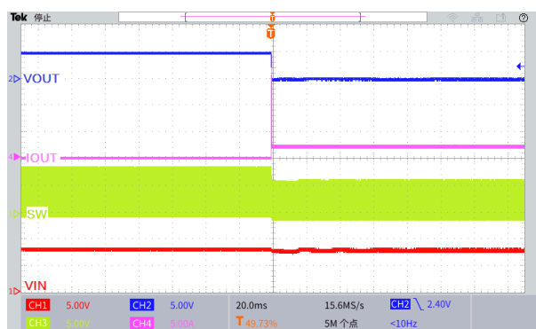
Figure21. Output Short Circuit Waveform ( V_{IN}=8V , V_{OUT}=5.0V )
